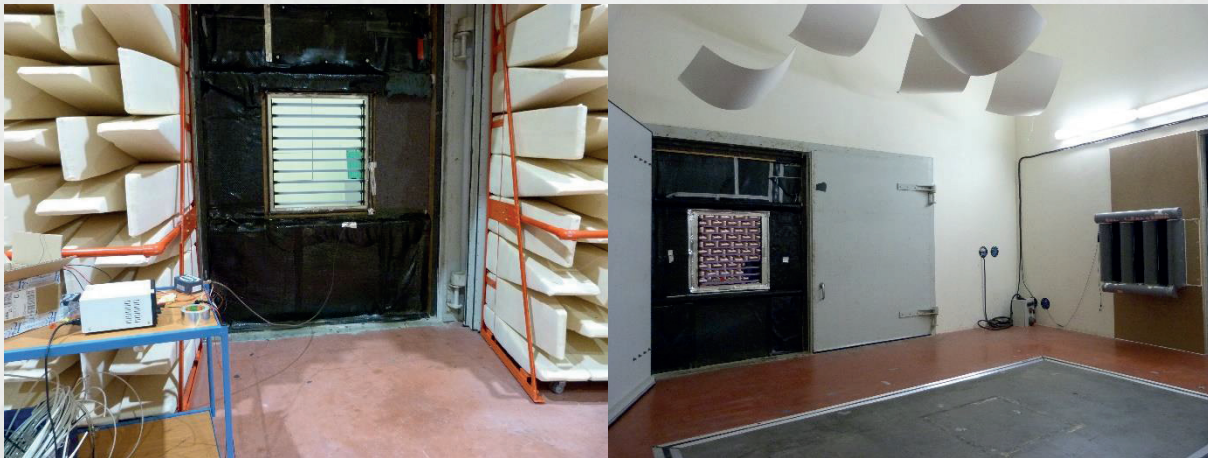
Photos 1 and 2: Sample seen from the semi-anechoic room (left) and the reverberant acoustic room (right)
